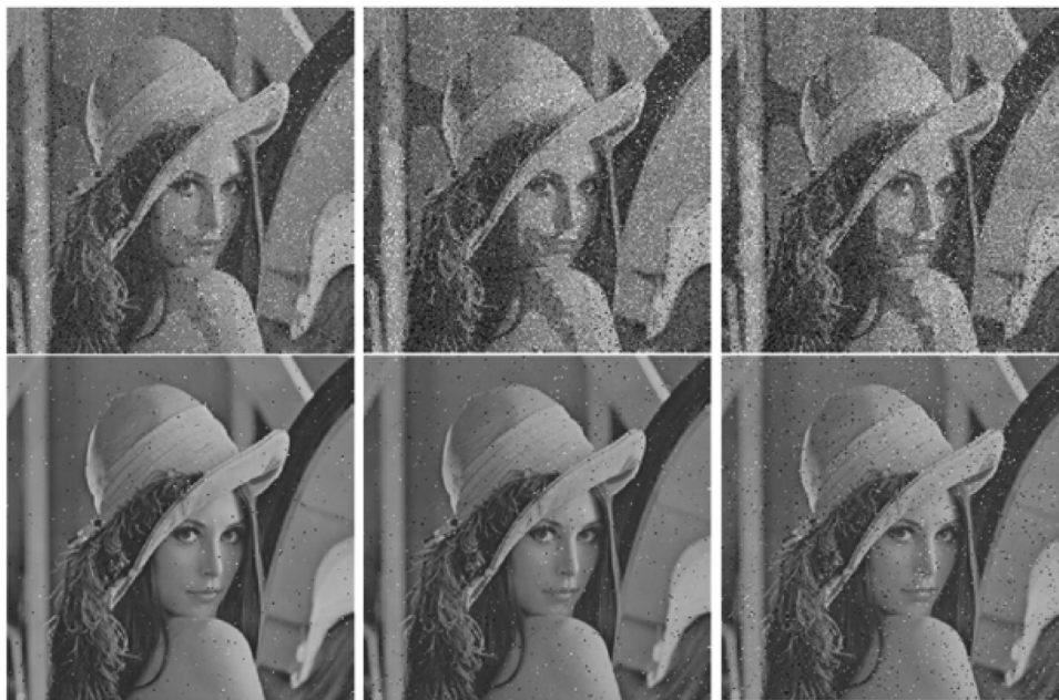
Fig. 10. Noise attacks of Lena image by different types of noise. Top row: restored images by adding Gaussian noise with variance 0.001, 0.005 and 0.01 on the cipher image, respectively; Bottom row: restored images by adding 1%, 2% and 5% salt-and-pepper noise on the cipher image, respectively.
