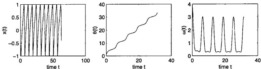
Figure 4. Left: the plot of the signal  $x(t) = \cos(t + 2 \arctan(\sin t / (2 - \cos t)) + ((2t + 1)/(t + 1)))$ . Middle: the phase of the signal  $x(t)$ . Right: the instantaneous frequency of the signal  $x(t)$ .
